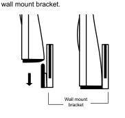
Or, if there is already a wall mount bracket installed, you can use a connector to align the brackets.
